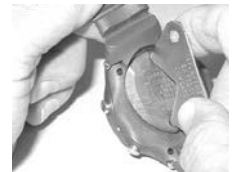
Fig. 126 - BATTERY Cover INSTALLATION
